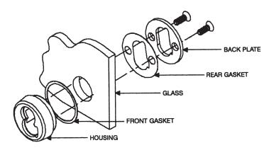
**Note:** Lock can be adjusted for use on different material thicknesses by using an "O" ring or changing the screw length. The 723S ships standard with 3 screw sizes (7/16", 3/4" and 1").
