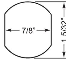
Lock diameter is 1-1/8". Drilled hole should be slightly larger.
