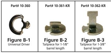
B-2 and B-3 drivers are based on use with standard Schlage compatible cylinders. If you are using a non-standard cylinder, you may need to modify the length of the B-2 or B-3 tailpiece to properly fit the cylinder into the lock body.
